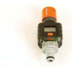
The water volumeter is plugged ontop of the intake connector. It has various programmes, which can be chosen by pressing the orange button. For the following described experiments it is always used the "liters per min" mode.
