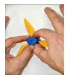
To replace the blades, a small nose is located at head of the hub. If the nose is pressed lightly on a hard surface, the hub-cap can be removed easily.
