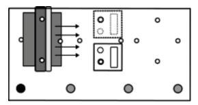
To measure the wind speed you have to remove the wind turbine from the base unit. Afterwards you plug in the holder for the wind measurement device as you can see in the sketch. For a more precise measurement you can calculate the average from the left and the right measuring point.
