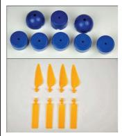
With the available components, rotors with 2, 3 or 4 blades and with a flat or an optimized profile can be created. There is a hub for 4 blades with a pitch angle of 25° and hubs for 3 blades with pitch angles of 20°, 25°, 30°, 50° and 90°.
