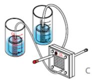
6. The electrolyzer can now be placed onto the module plate and be connected to it using the respective cables (red for  $O_2$ , black for  $H_2$ ).
