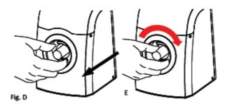
4. While the status light is flashing red, the H<sub>2</sub>-Storage is being filled. Only when the status light flashes green, the cartridge is completely filled. The stick may now be removed by turning it counter clockwise.
