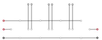
The base unit is a breadboard where up to 4 components can be plugged in a series and parallel connection. The current flows along the wires on the bottom side. At the head there are bypass slots to connect the components in the desired way.
