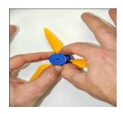
To replace the blades, a small nose is located on the head of the hub. If the nose is pressed lightly on a hard surface, the hub-cap can be removed easily.
