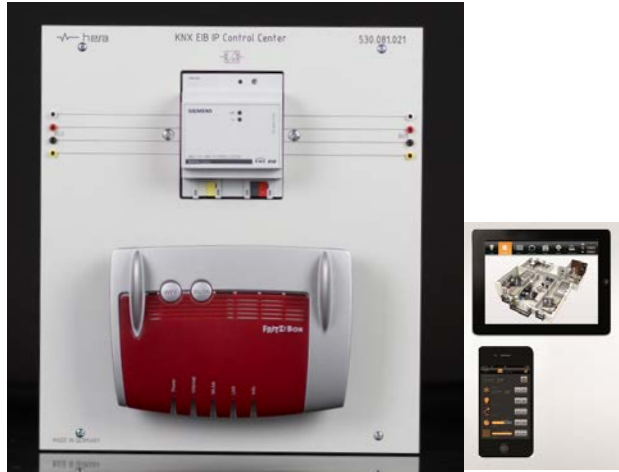
530.081.021 IP Control Center (W: 266) communication between KNX devices and computer (or e.g. smart phone) WLAN-Router Web-Server for control and monitoring (e.g. control by computer, smart phone or notebook) web-editor for creating a full graphic design with all control and monitoring elements
