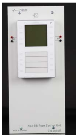
530.081.015 KNX EIB Room Control Unit (W: 133) control of heating, ventilation and air conditioning control of light, shutters and scenes temperature indication 16 programmable buttons
