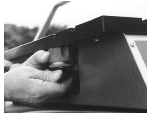
When a fresh reel of wire is needed on the bobbin, remove the remains of the original and thread the new wire into the small securing hole. Wrap the wire onto the bobbin and thread the end up through the table, making sure that it sits between the two aluminium pressure disks on the lower terminal. Form a loop in the new end and tension as in the previous paragraph.
