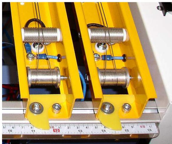
The workstop on the front table of the machine provides a fixed reference point for the edge of the material being formed. It can be fitted in either one of two positions, or at the rear of the machine, depending upon operator preference.
