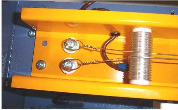
While holding the wire under slight tension, lay it across the grooved rollers and feed the end of it around the guide roller at the other end of the heater beam.
