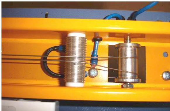
Attach the tensioning spring.
