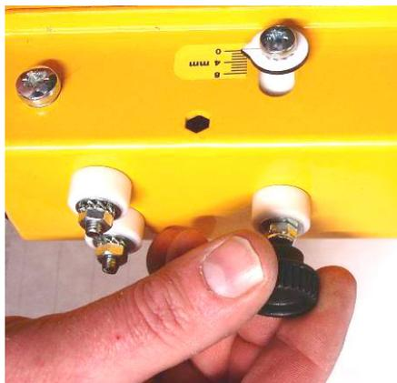
Use the adjusting knobs underneath each end of the heater beam. Looking from beneath, turning clockwise lowers the heating wires. Turning anti-clockwise raises the heating wires.
