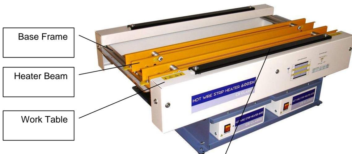
Workstop. Note that there are two sets of mounting holes for the workstop. The operator can choose which set are most appropriate depending upon the characteristics of the panel being produced.
