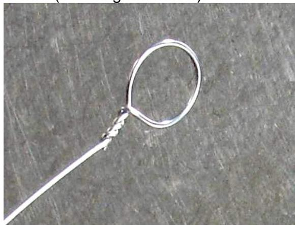
Fit the heating wire around the fixed post on the end of the heater beam.
