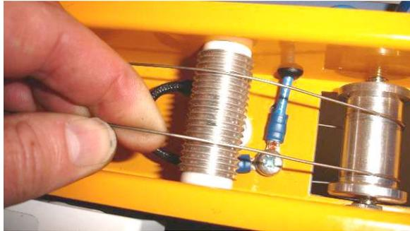
Ensure that the wires have cooled fully before handling. Lift the wire out of its groove, and position in the required groove
