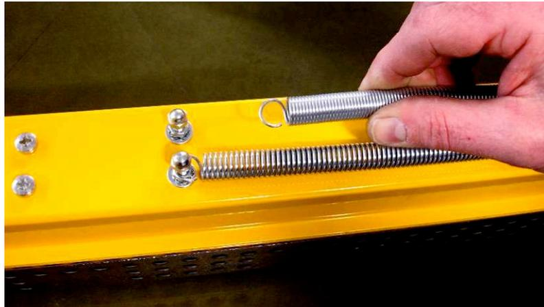
Unhook the tensioning spring from its securing post.
