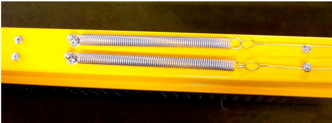
Please note that each heater beam will accommodate a maximum of two heating wires.
