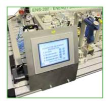
ENS-200 includes an HMI (Human Machine Interface) with a built-in PLC, interactive menus guide the user through the different activities.
