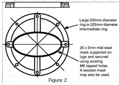
top of the dome to produce a concave base, (see Fig. 3). Note that success will be more certain if the supplied rings are relied upon to create the air seals and the fabricated masks only serve to modify the shape of the workpiece. Although this will inevitably involve some increase in material wastage, reliable air sealing does require precision and rigid clamping frames as supplied in the form of the cast aluminium units.
