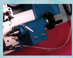
Manual Tailstock Steady Includes a rotating centre for supporting longer work pieces.
