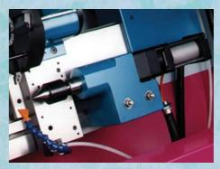
Automatic Pneumatic Tailstock Quill Includes a rotating centre and is interlocked and programmable. Ideal for use in FMS/CIM systems.
