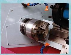
Automatic Pneumatic Chuck 3-Jaw closed centre chuck, interlocked and programmable. Can be controlled externally via optional robot port for FMS/CIM integration.
