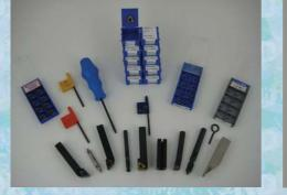
**Comprehensive Tooling Set** A package of external and internal tooling ideal for populating the 8 station turret. Includes a selection of spare inserts.
